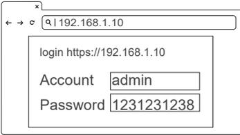
**STEP5/** Open a browser and enter IP Address 192.168.1.10 to login into the setup page. Use the following credentials to login.
