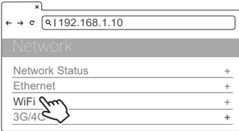
**STEP5/** Select the Wi-Fi and 3G/4G module to enter the setting.
