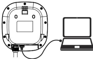
**STEP3/** Connect the RJ45 cable to the charger. Connect the RJ45 cable to the notebook.
