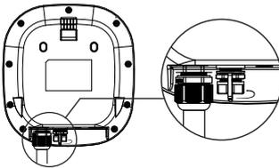
**STEP2/** On the bottom of the unit, you will find the RJ45 connector port knob. Turn the knob counterclockwise as shown on the left to open and access the RJ45 female connector.
