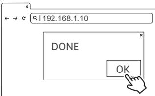
**STEP4/** After completion, click SET. Wait for the setting completion window to appear. Click "Confirm" to finish the setting. Restart the charger.
