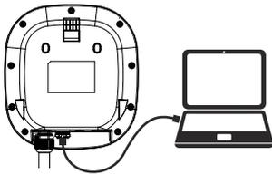
**STEP1/** Connect the RJ45 cable to the charger. Connect the RJ45 cable to the notebook.
