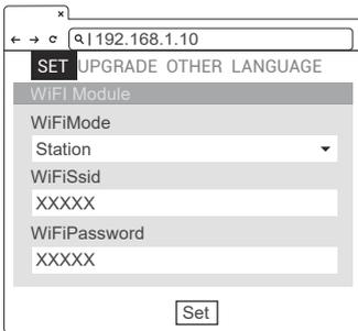
**STEP3/** Keep the Wi-Fi Mode set to "Station" and enter the Wi-Fi SSID name and the Wi-Fi password. Save settings by selecting SET.
