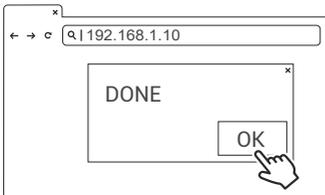
**STEP4/** After completion, click SET and wait until the setting completion window appears. Restart the charger.
