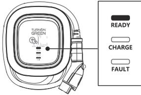
**STEP1/** After power-on, the green (READY), blue (CHARGE), and red lights (FAULT) will all light up. The charger will then enter standby mode, and the green light (READY) will remain lit. This could take up to 90 seconds.
